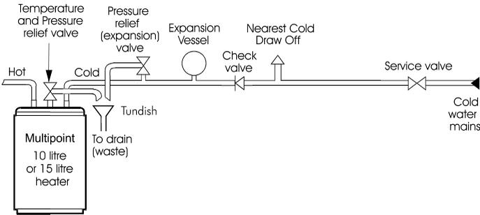
**Diagram 3** For inlet water pressures above 4.1 bar (60 p.s.i.)
